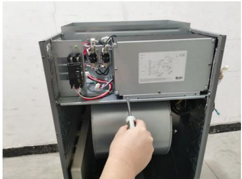
10. Reinstall the front and upper panel to the air handler to complete the installation process.
