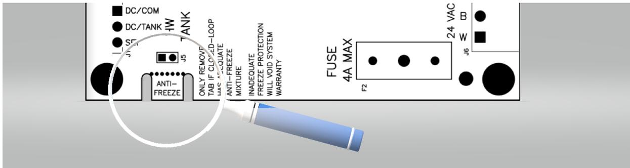
**IMPORTANT!!!** Once the tab has been removed, the unit will permanently be set to 20 degrees and cannot be reversed!! Removal of the tab on open loop systems or closed loop systems without minimal freeze protection will VOID all warranty on the unit!
