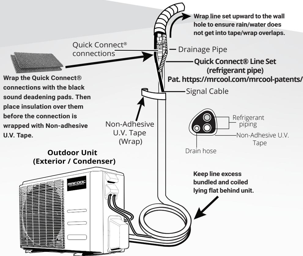
1. Pack the wall hole with the supplied Neoprene (or Spray Foam), filling any space not taken up by the piping & lines, in order to seal the hole.
