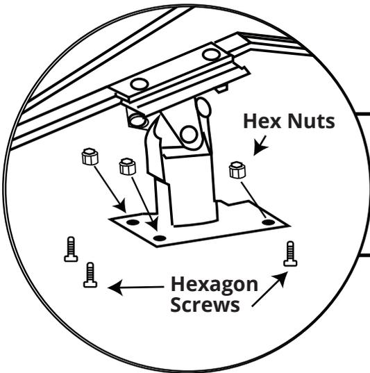
**After installing the transition fitting, attach the motor component to the bottom plate using hex nuts and hexagon screws. Tighten the screws to complete installation.**
