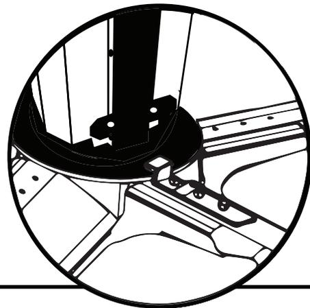
According to the diagram, use the aluminum fan base and safety plate to clamp the fan blade components to the middle position, and then pass through the screws to secure them.
