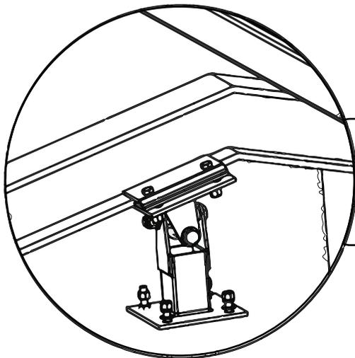
According to the diagram, install the transition fitting on the steel I-beam, and then lock the fastening screws to complete the installation.
