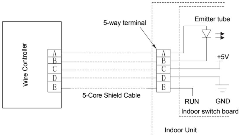
When a wire controller is needed, a small 5-way terminal should be added, fix an infrared emitter with gumwater near the receiver on the switch board. Connect its anode and cathode to A and B, and +5V, GND, RUN to C, D, E on the switch board.
