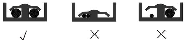
Use the specified electric wire. Connect the wire securely to the terminal. Lock the wire down without applying excessive force to the terminal. (Tightening torque:  $1.31\text{N.m} \pm 10\%$ ).
