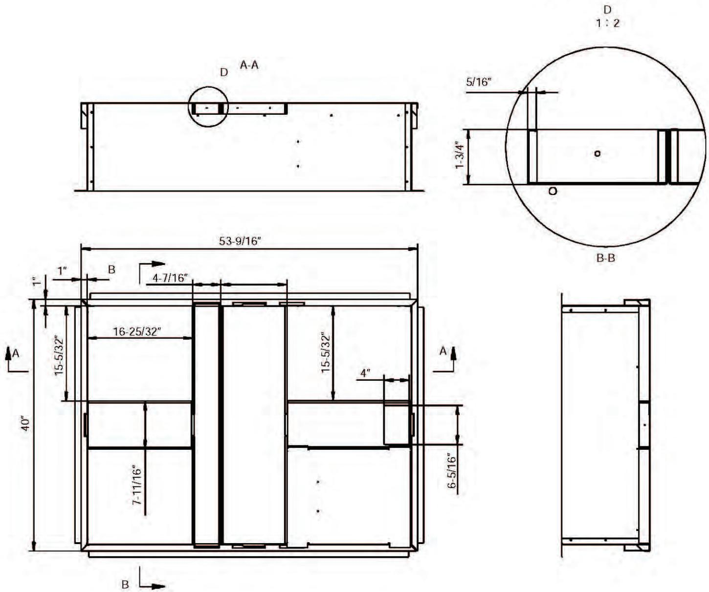
**Fig.3-7 Roof Curb Details**
