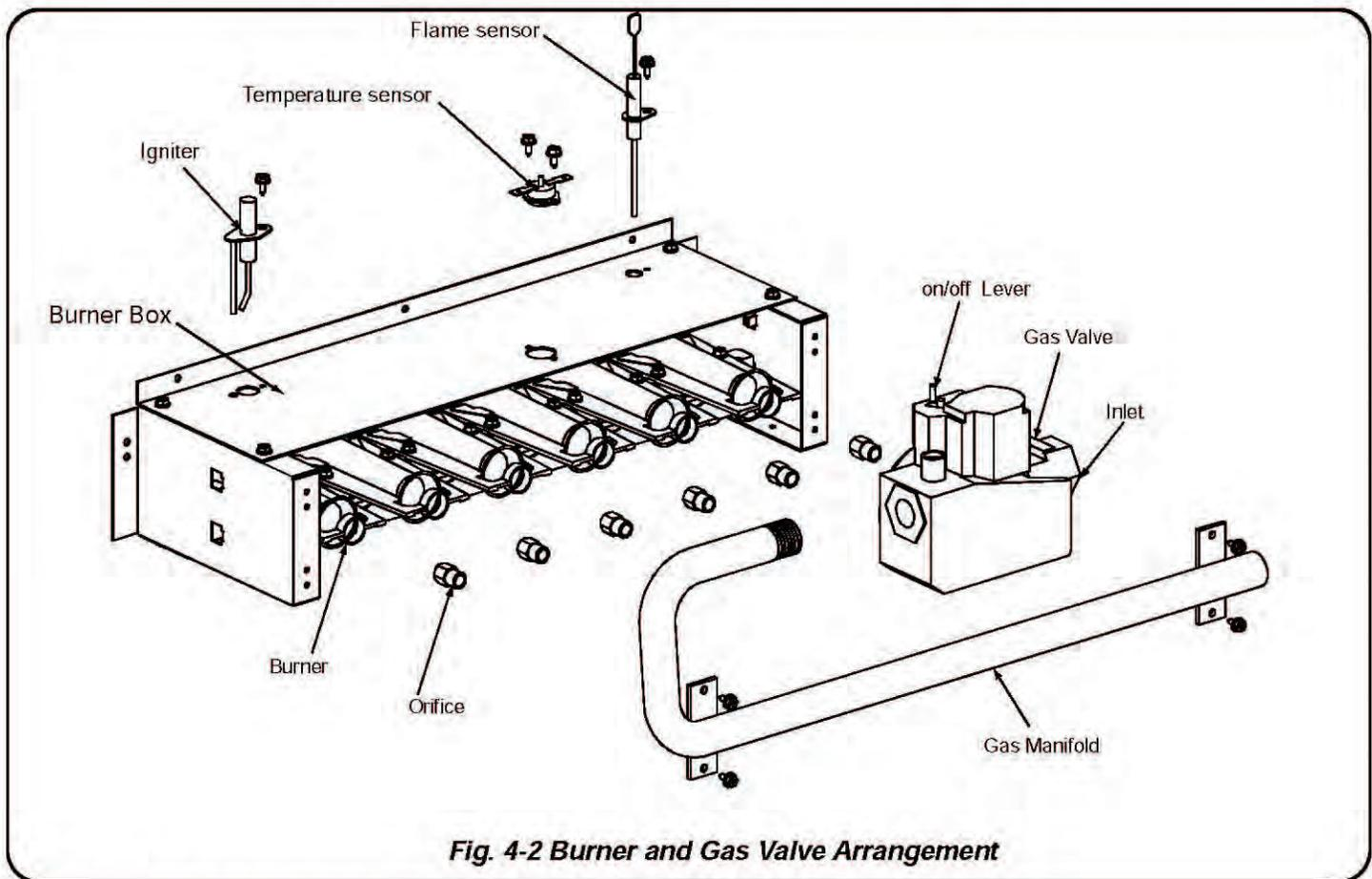
**Fig. 4-2 Burner and Gas Valve Arrangement**
