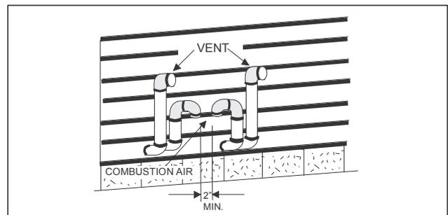
**Fig 23:** Double Horizontal Combustion Air Intake and Vent Termination
