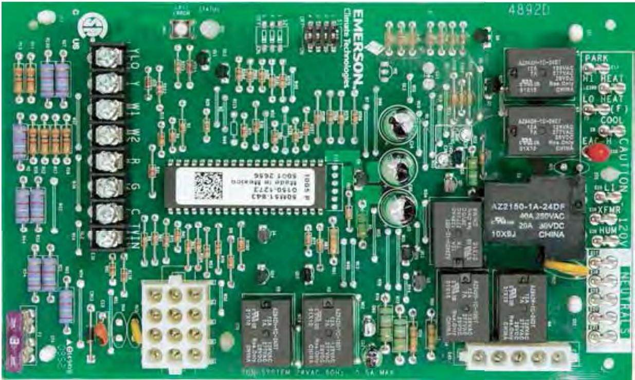
Fig. 32 - Furnace Control
