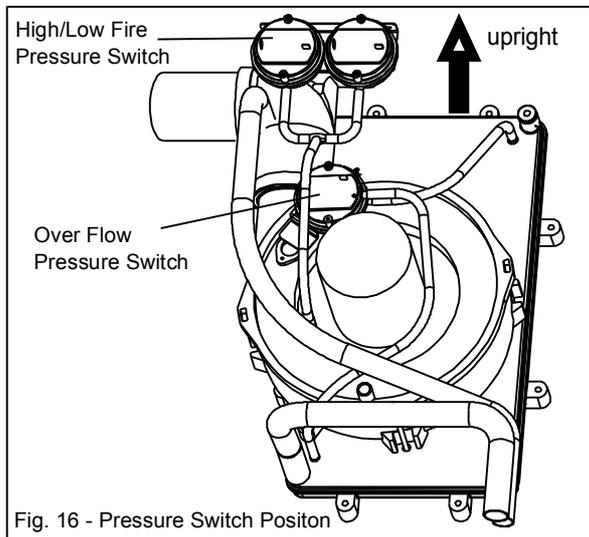
Fig. 16 - Pressure Switch Position
