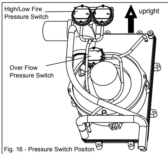
Fig. 16 - Pressure Switch Position
