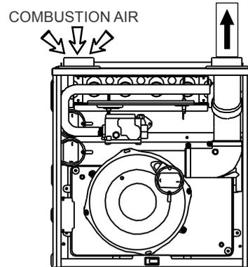
Fig 26: Combustion Airflow Path Through The Furnace Casing
