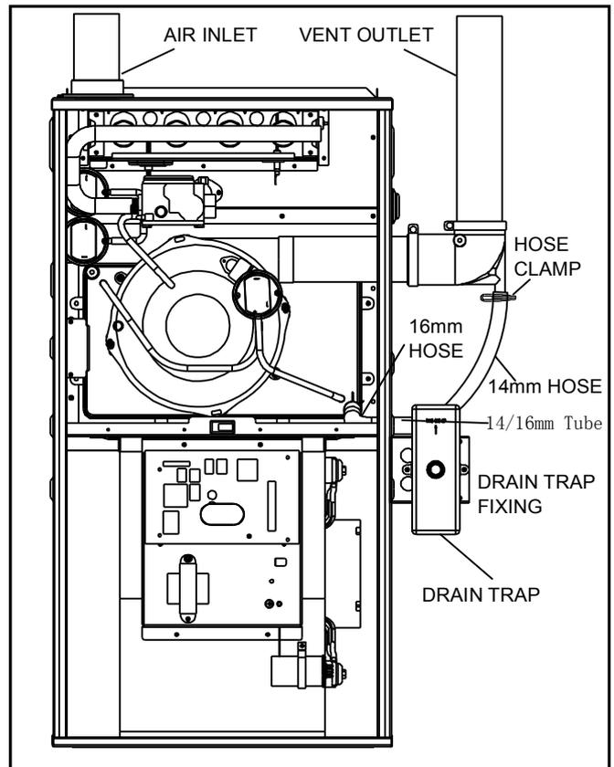
Fig. 12 - Upflow Installation, Right Side Venting
