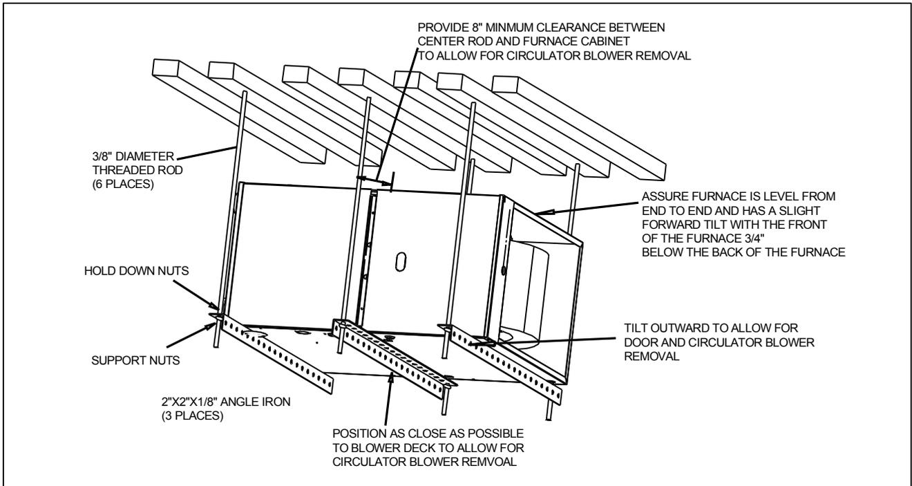
Fig. 8 - Horizontal Installation
