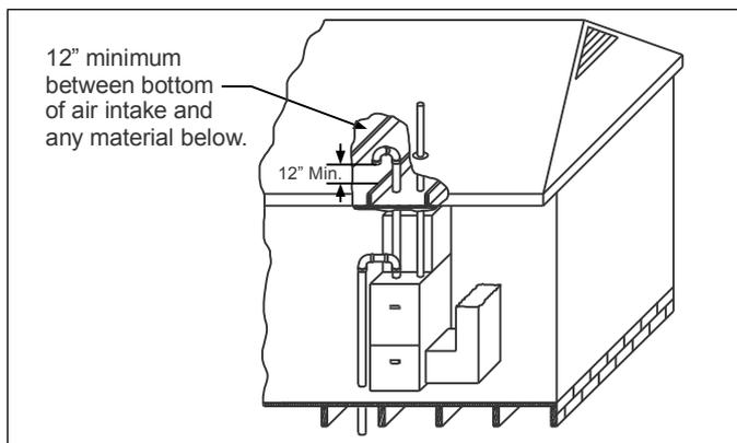
**Fig 28:** Attic and Crawl Space Combustion Air Termination
