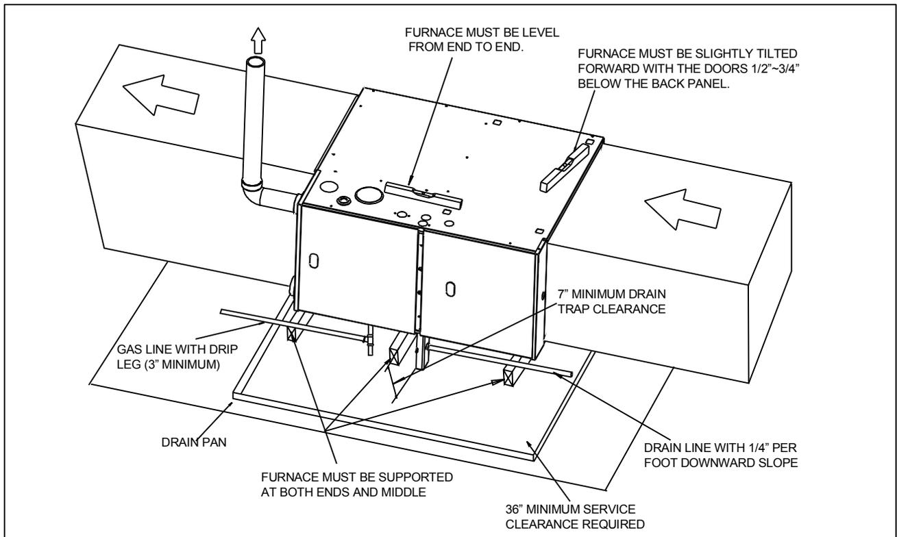
Fig. 9- Horizontal Installation
