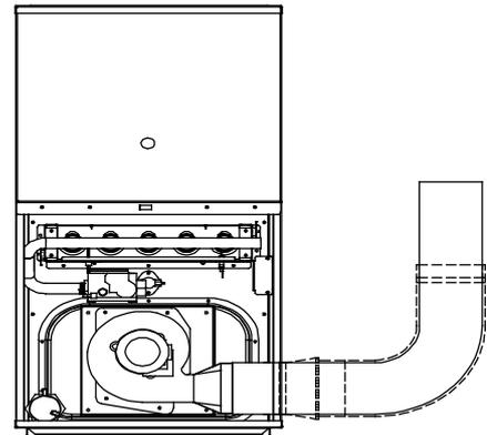
Fig. 13- Downflow Application- Vent Elbow Up then Right
