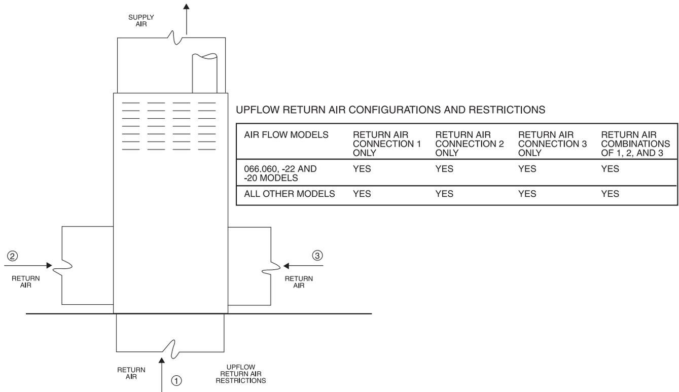
Fig. 18 – Upflow Return Air Configurations and Restrictions
