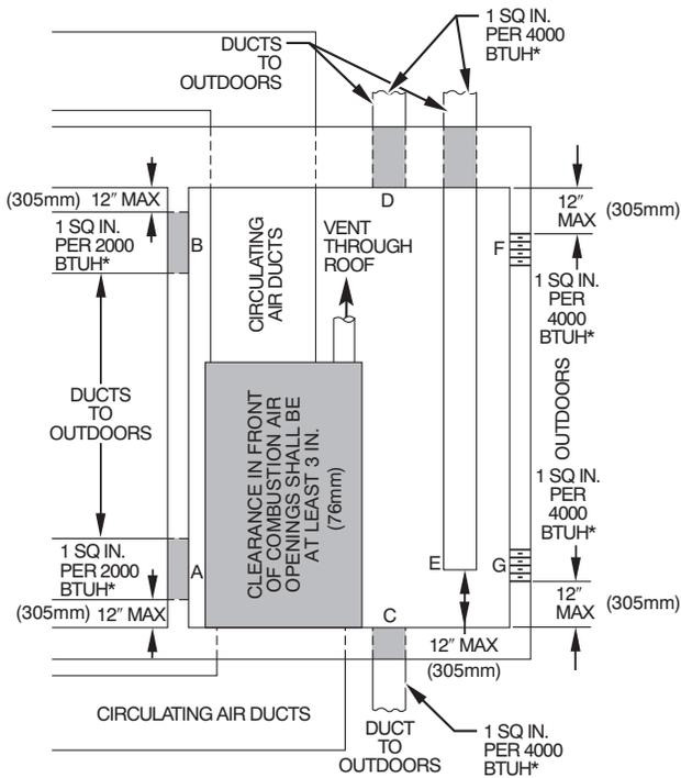
\*Minimum dimensions of 3-in. (76 mm).
