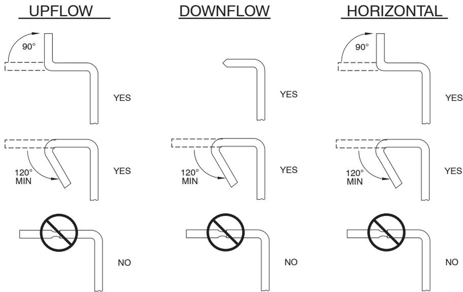
**Fig. 14 - Duct Flanges**
