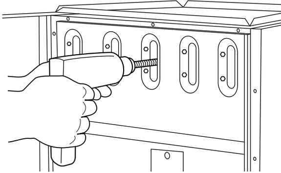
**Fig. 48 – Cleaning Heat Exchanger Cell**
