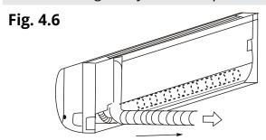
3. Now, you will need to lightly tape the refrigerant piping and drain pipe together in a bundle, using electrical tape, making sure that the drain pipe is at the bottom. *DO NOT* tape the ends of the piping (connectors). Refer to Fig 4.7 and the image below for the correct orientation of the piping when taping.
