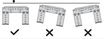
NOTE: Use a level in order to ensure your mounting plate is mounted to the wall with the correct orientation shown above.
