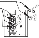
A: Low pressure stop valve B: High pressure stop valve C & D: Indoor unit flare nuts
