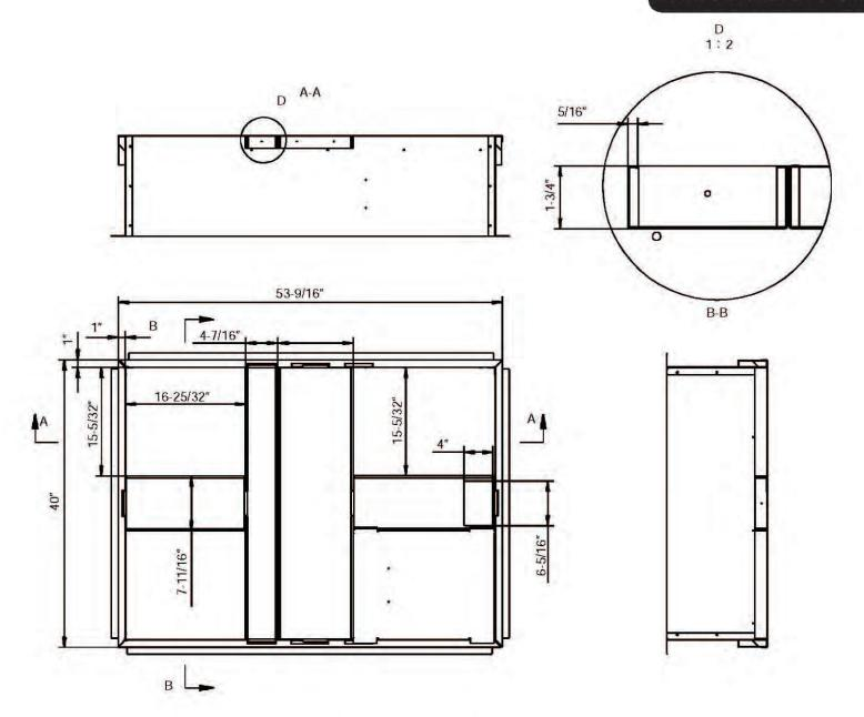
Fig.3-7 Roof Curb Details
