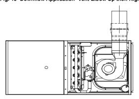
Fig. 15 -Horizontal Right Application-Vent Elbow Up
