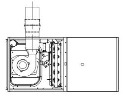
Fig. 14 -Horizontal Left Application-Vent Elbow Up
