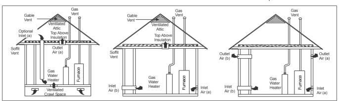
Fig. 22 Outside and Ambient Combustion Air
