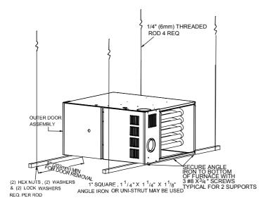
Fig. 9 - Horizontal Unit Suspension
