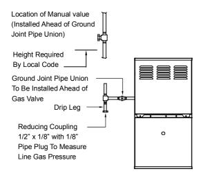
Fig. 24 - Typical Gas Pipe Arrangement
