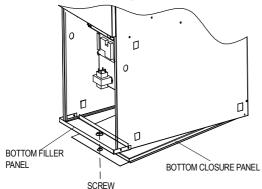
Fig. 5 - Removing Bottom Closure Panel
