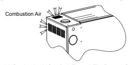
Fig. 21: Combustion Airflow Path Through The Furnace Casing to the Burner Box
