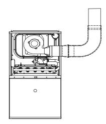
Fig. 18 -Upflow Application-Vent **Elbow Right**
