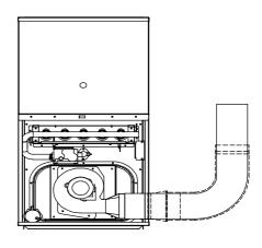
Fig. 13- Downflow Application- Vent Elbow Up then Right
