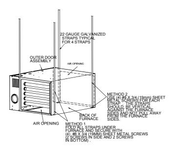
Fig. 10 - Horizontal Suspension with Straps
