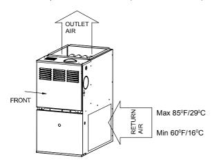
Fig. 3 - Return Air Temperature
