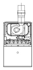
Fig. 17 -Upflow Application-Vent **Elbow Up**
