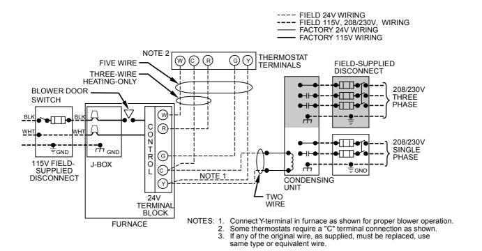
Fig.27 - Heating and Cooling Application Wiring Diagram with I-Stage Thermostat
