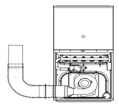
Fig. 12 - Downflow Application- Vent Elbow Up then Left
