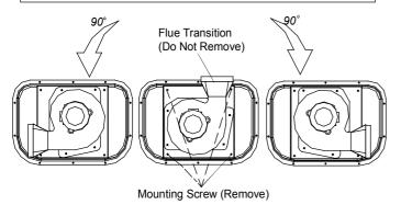
Fig. 20 Combustion Air Inducer
