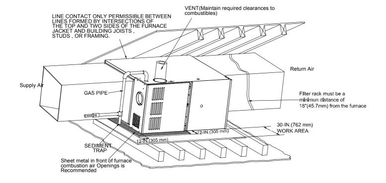
Fig. 11 - Typical Attic Installation
