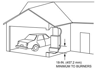
Fig. 4 - Installation in a Garage
