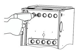
Fig. 34 - Cleaning Heat Exchanger Cell
