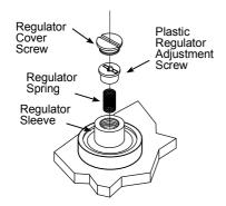
Fig. 28 Gas Valve and Regulator Adjustment
