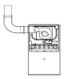
Fig. 16 -Upflow Application-Vent Elbow Left
