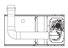
Fig. 38 - Horizontal Right Application-Vent Elbow Right
