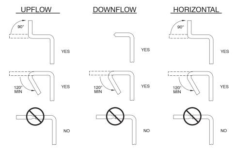
Fig. 14 - Duct Flanges
