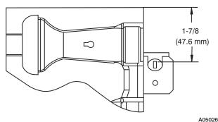
Fig. 47 - Igniter Position-Top View
