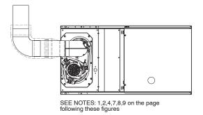
Fig. 34 - Horizontal Left Application-Vent Elbow Left
