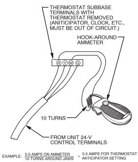
Fig. 44 - Amp. Draw Check With Ammeter
