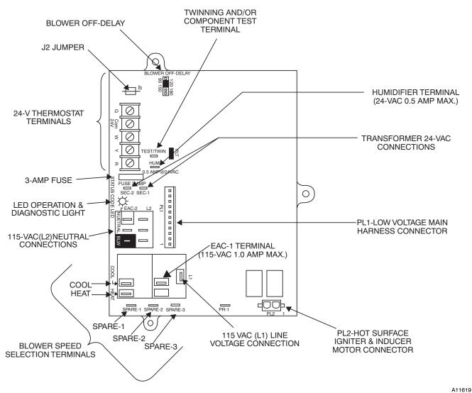
Fig. 25 - Furnace Control
