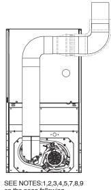
Fig. 33 - Downflow Application-Vent Elbow Up then Right
