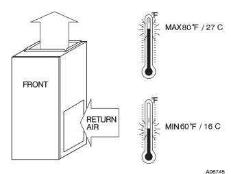
Fig. 3 - Return Air Temperature
