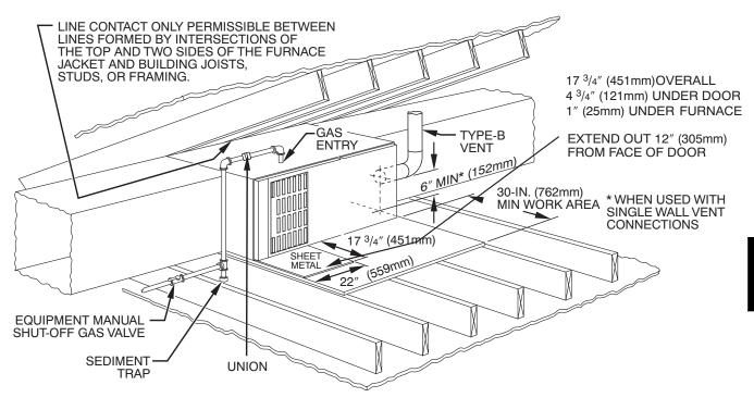
Fig. 17 - Typical Attic Installation
