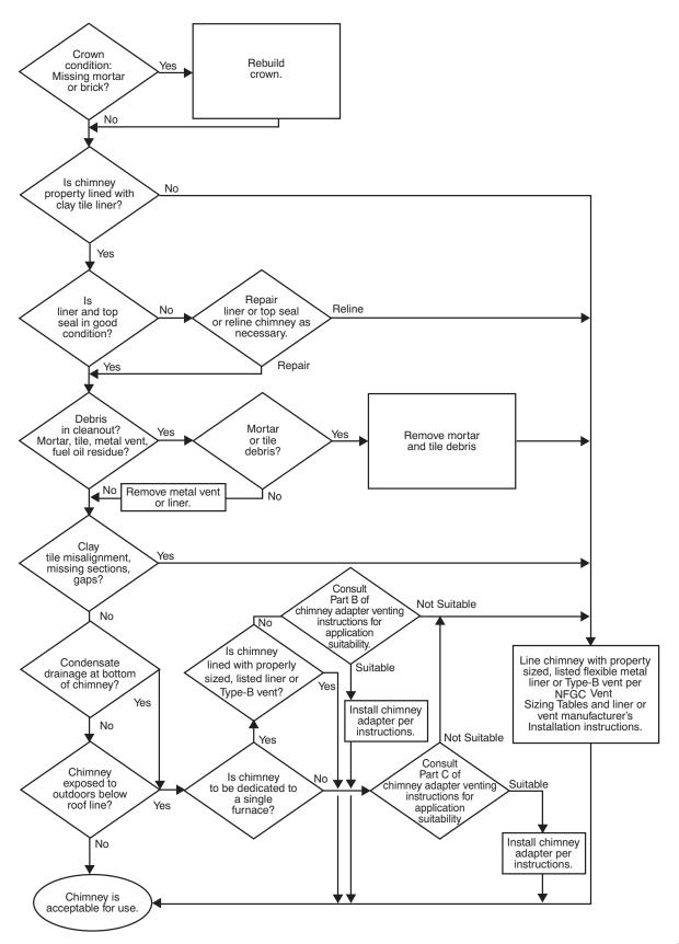
Fig. 27 - Chimney Inspection Chart
