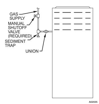
Fig. 22 - Typical Gas Pipe Arrangement
