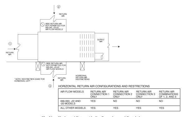
Fig. 20 - Horizontal Return Air Configurations and Restrictions
