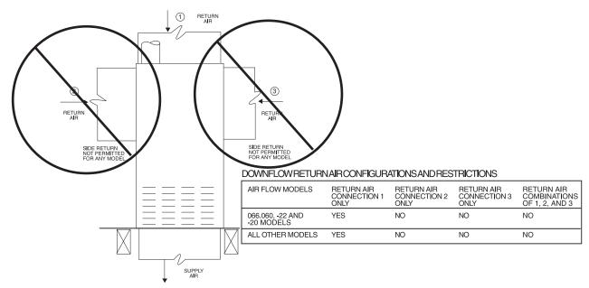
Fig. 19 - Downflow Return Air Configurations and Restrictions
