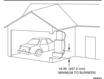
Fig. 5 - Installation in a Garage
