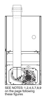
Fig. 31 - Downflow Application-Vent Elbow Up
