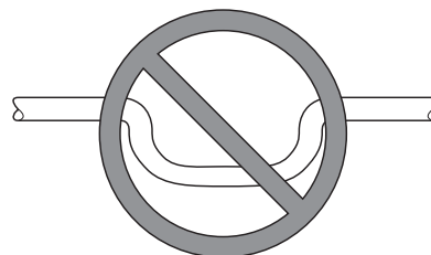
Fig. 20 - Insufficient Condensate Trap
